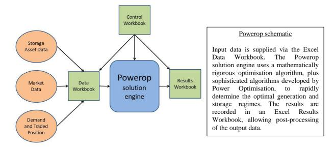
Powerop provides the results of each run via its Excel interface, allowing users to examine the optimised generation and storage regimes, trading activity, costs and revenues in detail.
